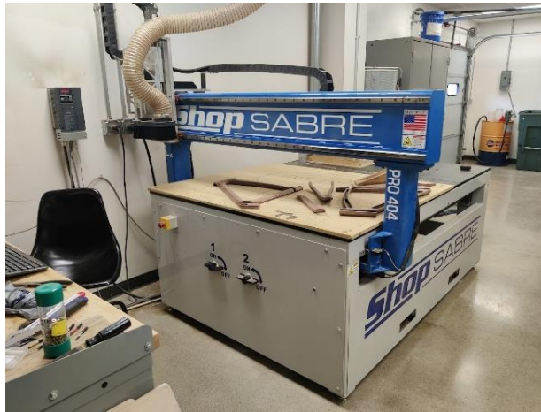
Figure 2.2.3. Shop Sabre CNC plasma cutter.
