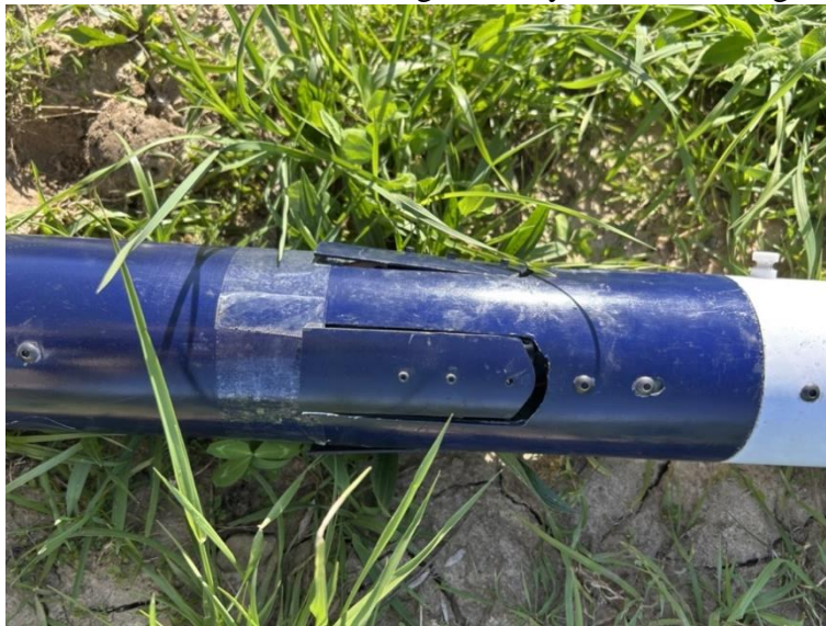
Figure 2.2.1. Image of the airbrake airframe slots after recovery of launch vehicle.
