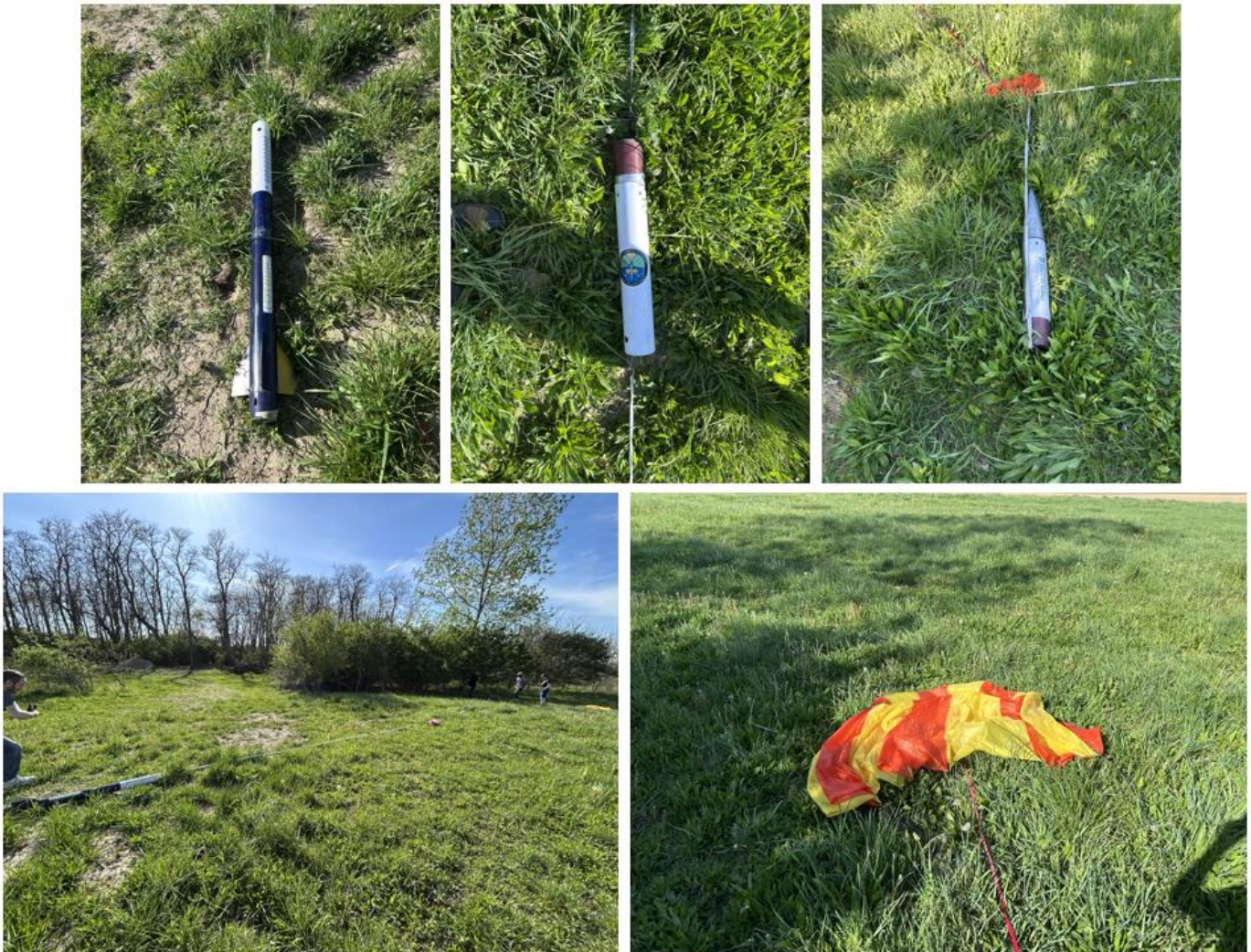
Figure 2.3. Landed condition of the independent sections of the rocket. All parts remained tethered during recovery.
