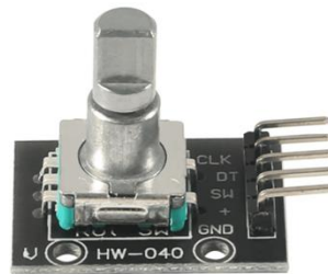
Figure 3.7.21. Rotary displacement sensor selected for the AB.
