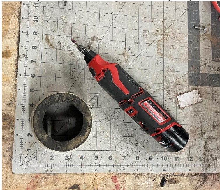
Figure 3.4.18. Electrical Dremel tool used to bore larger nozzle diameter
