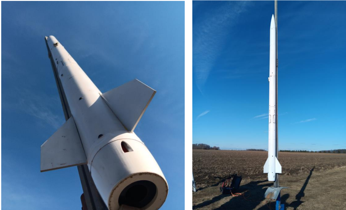
Figure 5.1.1. Chariot on loaded on launch rail for inaugural flight. Note the packing tape holding the airbrake flaps on from both the inside and outside of the airframe.
