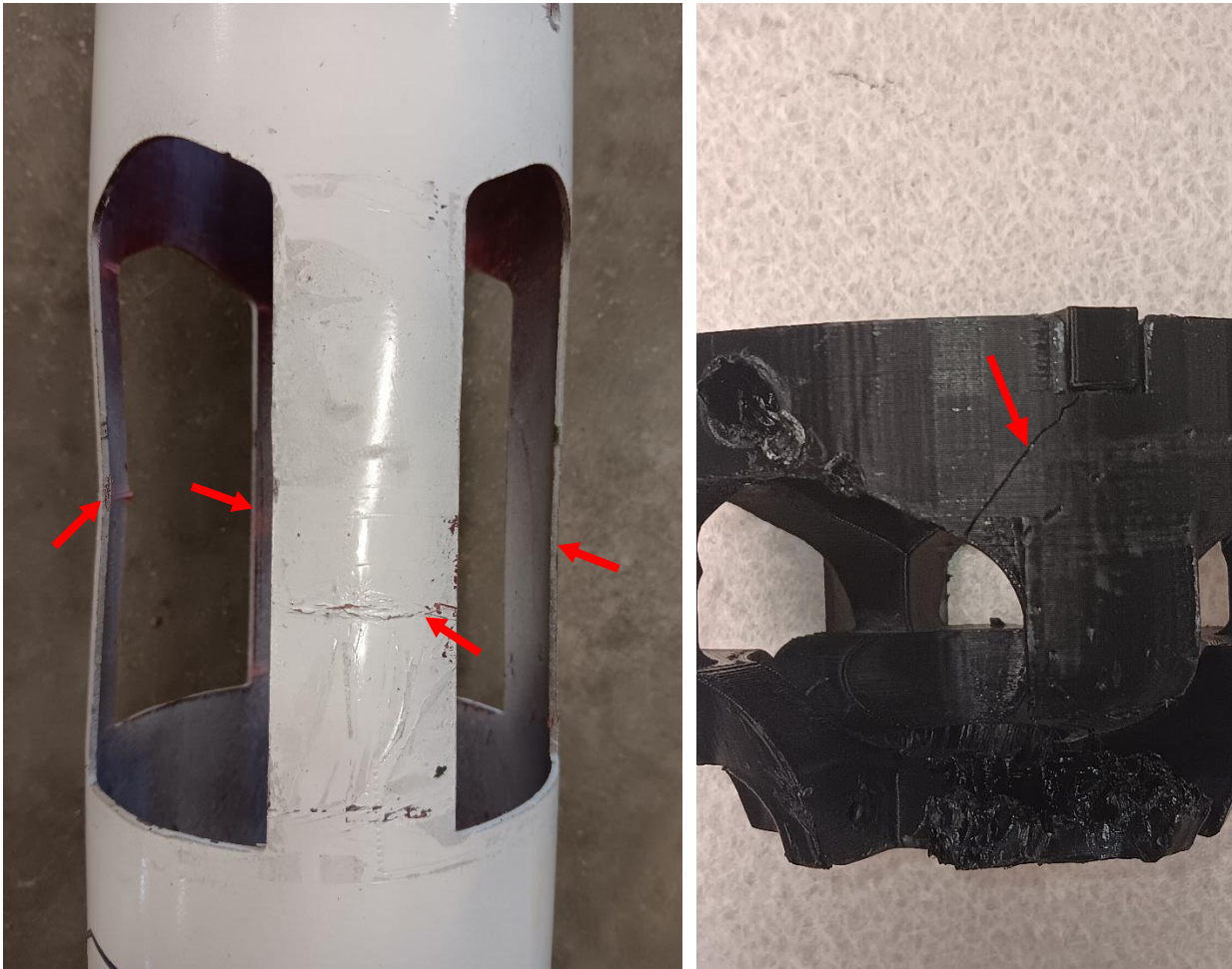
Figure 5.1.7. (Right) Damaged portion of the airframe after landing. All four of the stringers buckled to the point un-flightworthiness. (Left) Fissure in the airbrake encoder mount caused by the booster flexing upon landing. (Note: The rest of the damage to the part was a result of the airbrakes being broken out of the airframe and was not a result of the flight).
