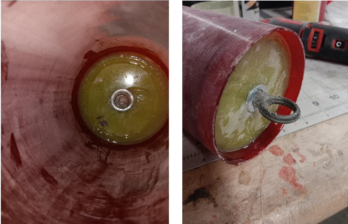
Figure 3.4.13. View of the interior and exterior fillets on the payload bay bulkhead.
