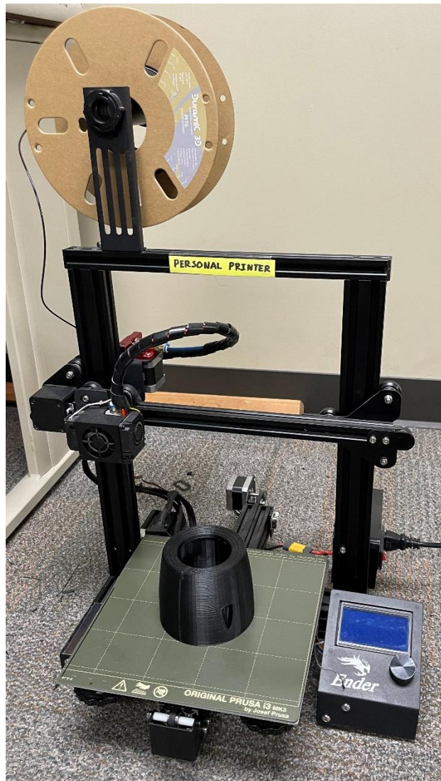
Figure 3.4.17. Ender3 printer used to print PETG tail cone, with finished cone for scale.
