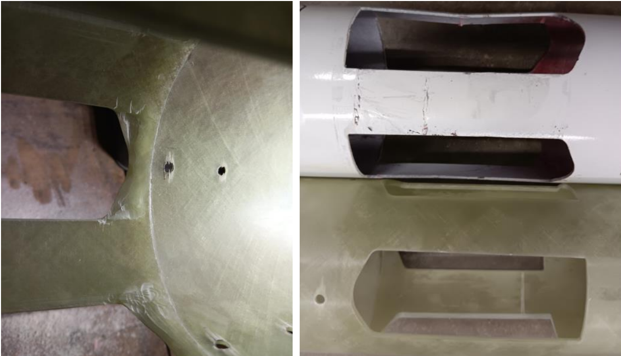
Figure 3.4.5. (Left) Interior view of the strengthening coupler added to the stringers; (Right) Comparison photo between the damaged airframe and the reinforced airframe.
