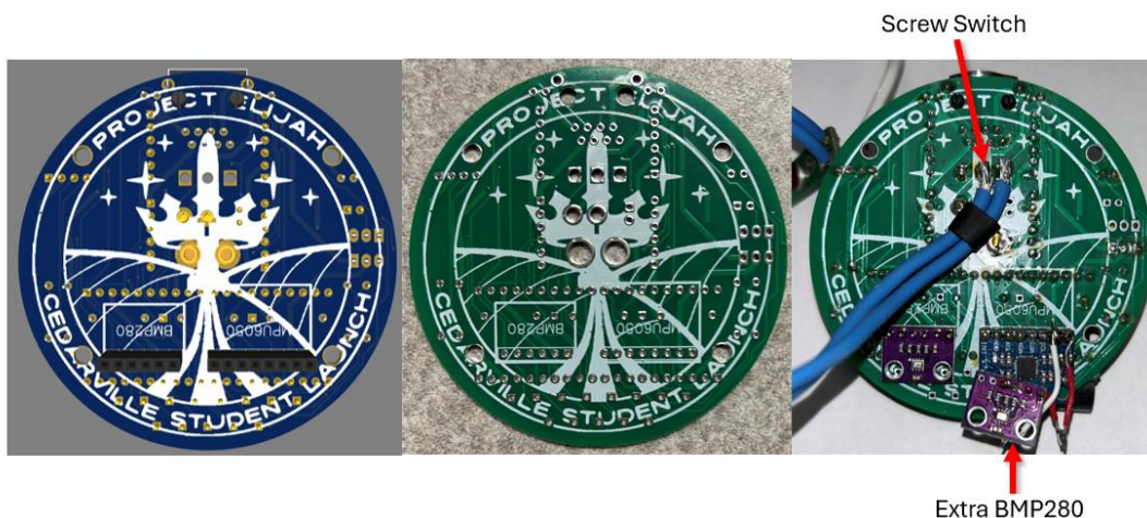
Figure 4.2.16. Bottom of Airbrakes PCB from EasyEDA to non-soldered to soldered.
