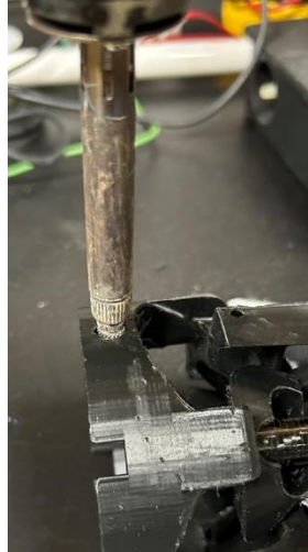
Figure 4.2.7. Process of inserting heat set inserts.
