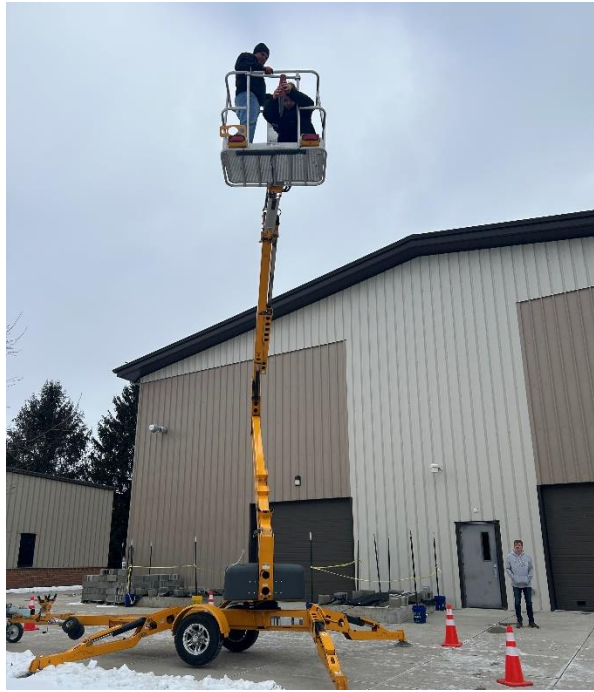
Figure 7.1.1. Drop test setup for maximum allowable kinetic energy at impact.
