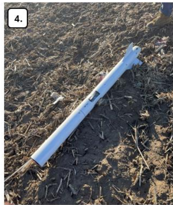
Figure 5.1.6. Close view of each of the free portions of the rocket after landing. Pictured are: 1) the broken tip of the 3D printed nose cone, 2) the payload bay, 3) the avionics section, and 4) the aft section of the rocket with the airbrake flaps detached and lying beside the rocket.
