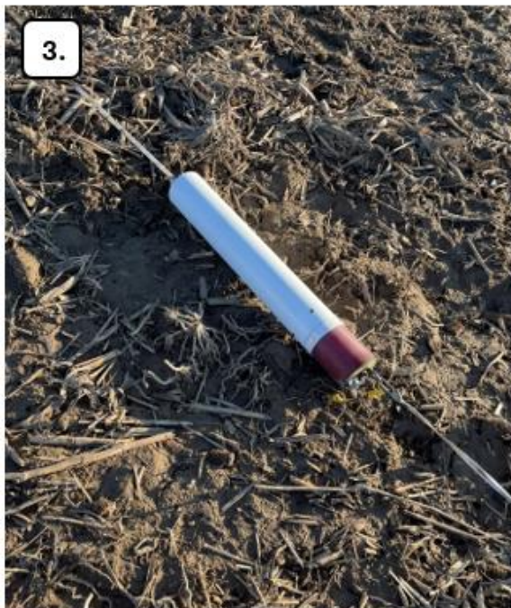
Figure 5.1.6. Close view of each of the free portions of the rocket after landing. Pictured are: 1) the broken tip of the 3D printed nose cone, 2) the payload bay, 3) the avionics section, and 4) the aft section of the rocket with the airbrake flaps detached and lying beside the rocket.
