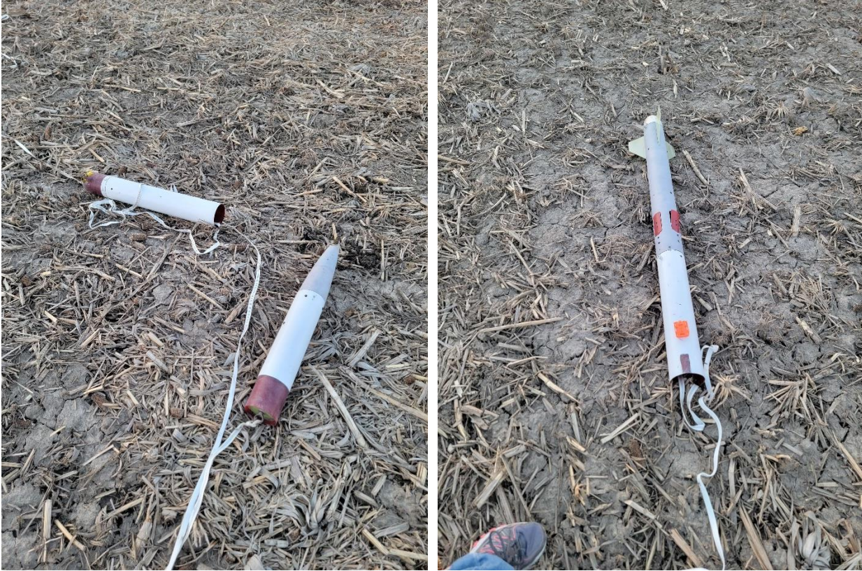
Figure 5.2.5. (Left) Close view of the payload bay and avionics section of the rocket; (Right) Aft section of the rocket. Note that the orange bracket that held on to the RunCam was empty upon landing.
