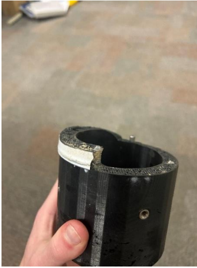
Figure 7.1.3. Damage to full scale cone indicating break above reinforcement pins.
