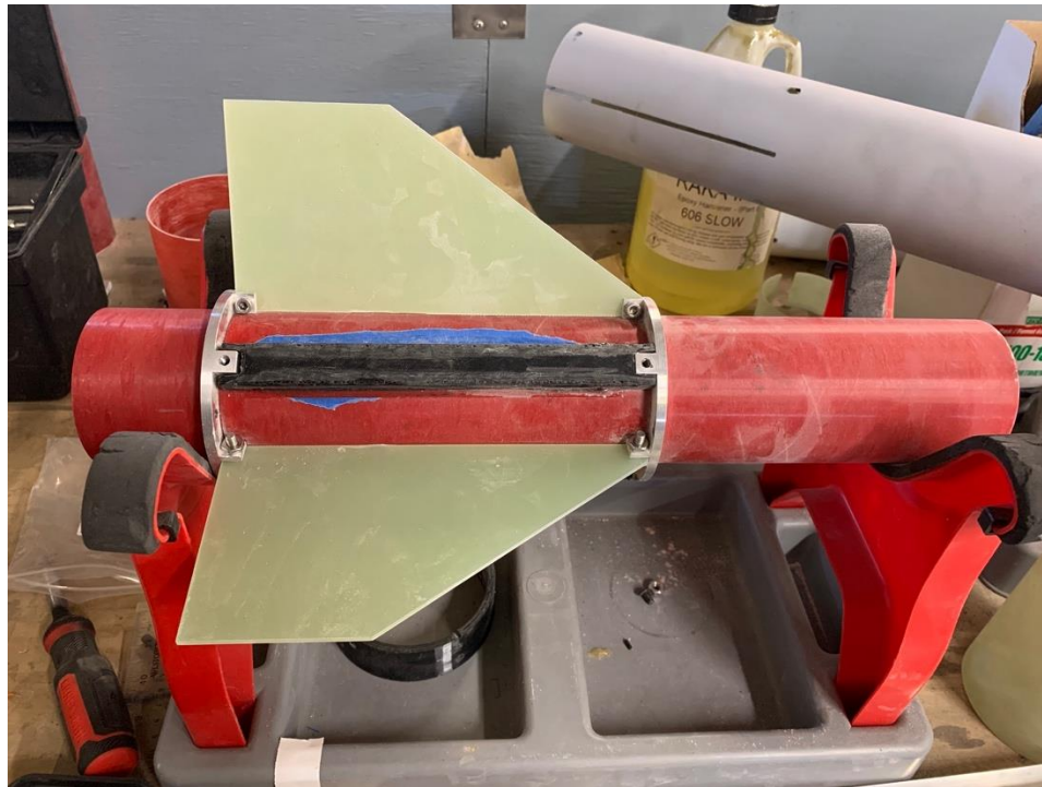
Figure 3.4.15. Centering rings, flanges, and fins securely fastened within the motor retainment system.
