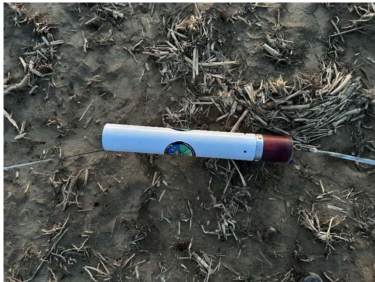
Figure 3.4.5. Chariot avionics section as landed configuration.
