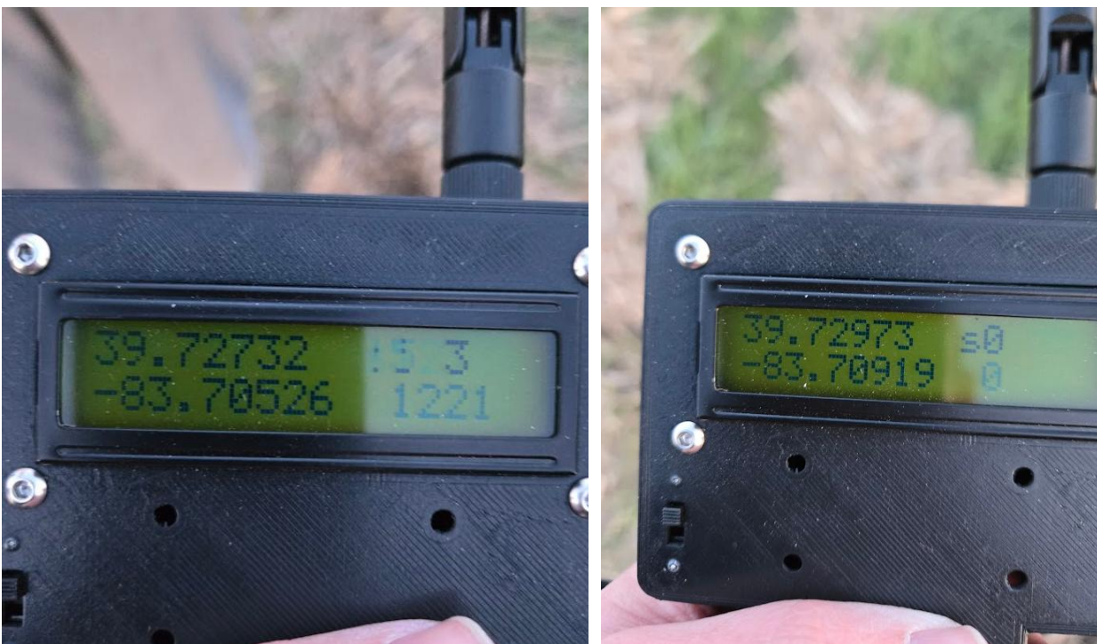
Figure 3.4.2. (Left) Picture of Eggtimer gps reciever while Chariot is on the launch rail. (Right) Eggtimer gps receiver after landing.
