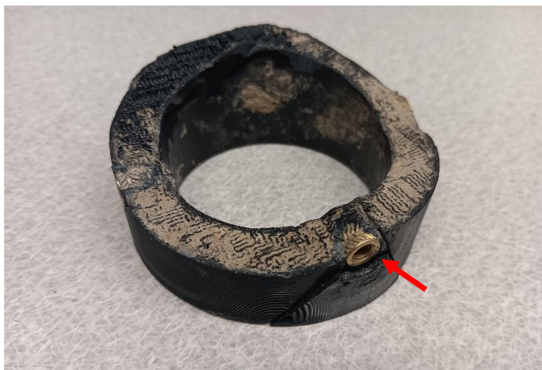
Figure 3.9.12. Nose cone failure point focused at the heatset inserts.
