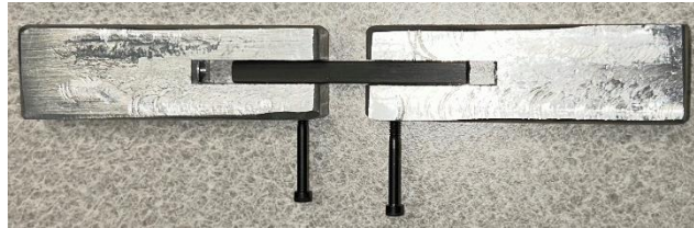
Figure 3.7.16. Tensile test apparatus before the test commenced.
