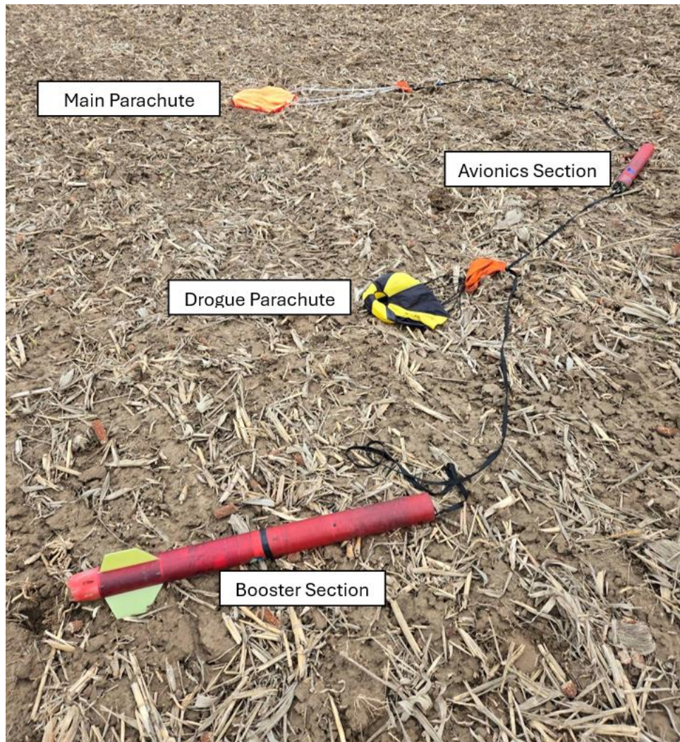
Figure 3.9.6. Landing orientation of the tethered subscale rocket pieces. The forward section of the rocket that separated during recovery is not shown in this picture.
