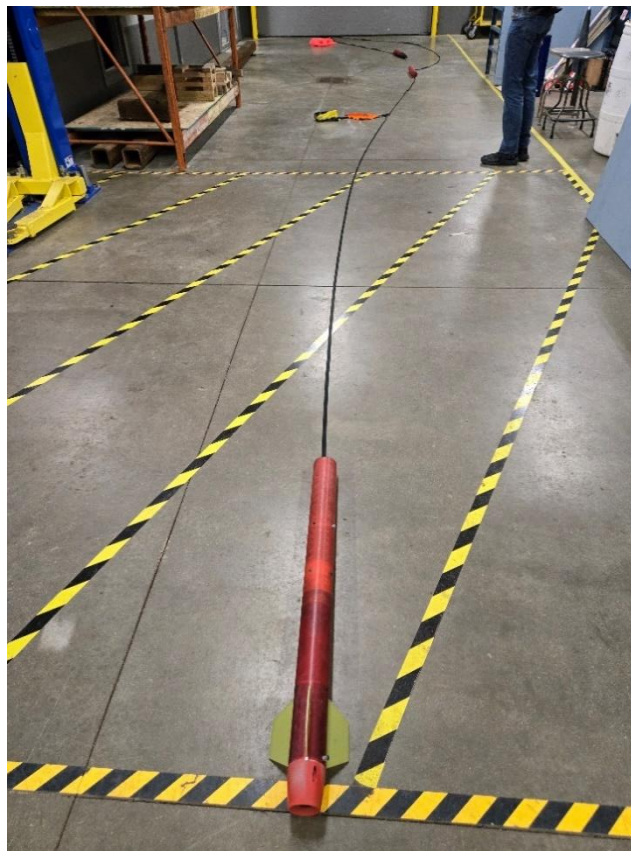
Figure 3.9.2. View of the subscale rocket spread out to ensure the rocket sections do not collide while under parachute due to improper shock cord length.
