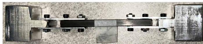
Figure 3.7.20. Compression buckling test on the coupler.
