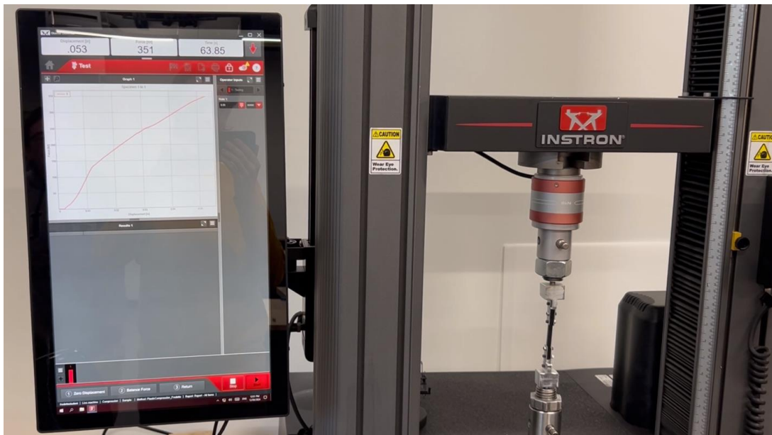
Figure 3.7.21. Compression test of the full coupler link and gusset connector plates in the INSTRON machine.
