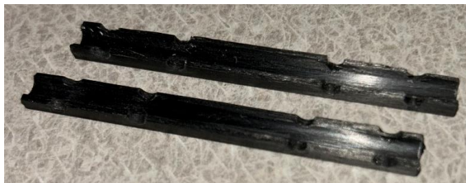
Figure 3.7.15. Failure in the coupler due to fiber reinforced anisotropic delamination.
