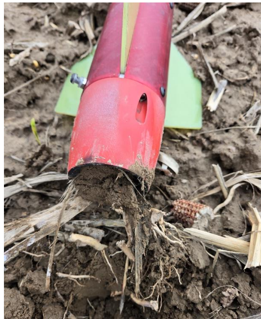
Figure 3.9.7. Aft end of the booster section. Note the surprisingly minimal charring due to exhaust.
