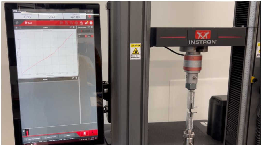
Figure 3.7.17. Tensile test of coupler link in the INSTRON machine.
